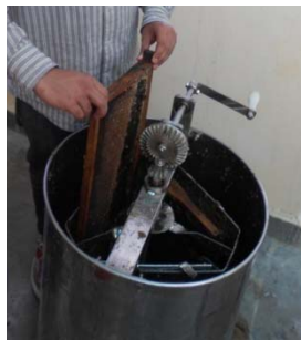
Placing uncapped honey combs in tangential honey extractor
